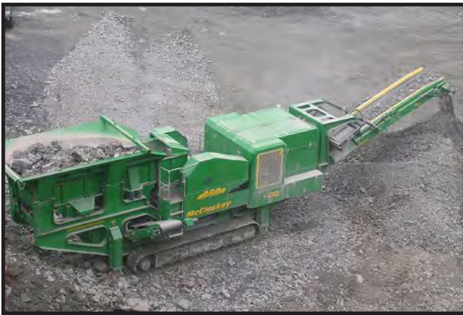
A McCloskey C44 (above) and a J50 (left) produce four grades of aggregate from stone transported to the crushing site.
