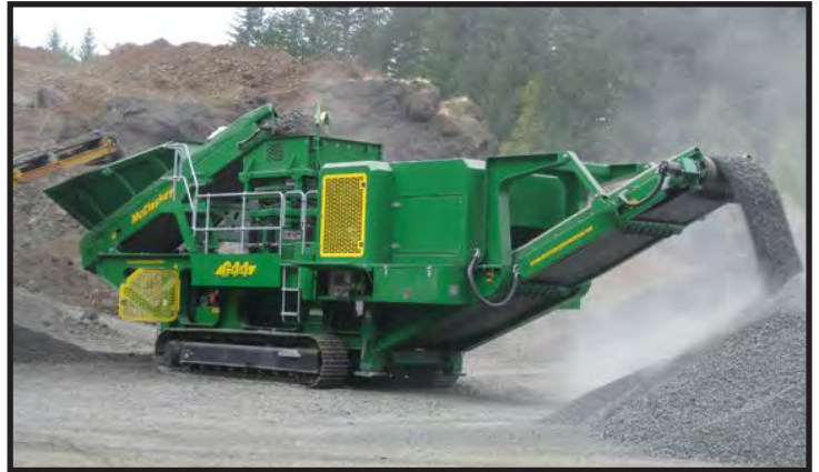
A McCloskey C44 (above) and a J50 (left) produce four grades of aggregate from stone transported to the crushing site.
