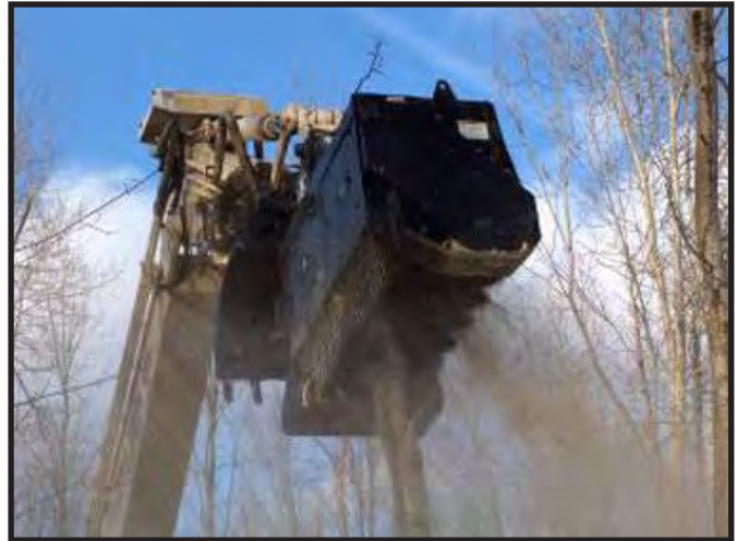
An excavator-mounted grinder reduces a standing tree to mulch.
